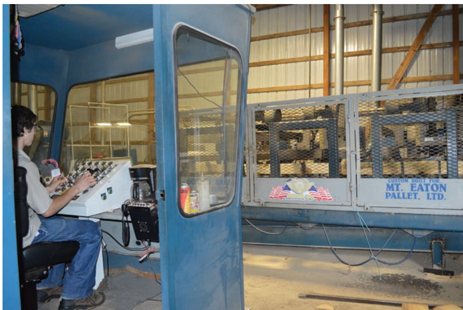
Mt. Eaton replaced its thin-kerf sawing system with its Brewer circular blade sawing lines because it gets better quality finished lumber, eliminating bearded lumber and sawdust on the boards. With their thin-kerf system their experience was that sawdust from frozen cants in the middle of the winter freezes back to the boards before you can get them to the deduster.
