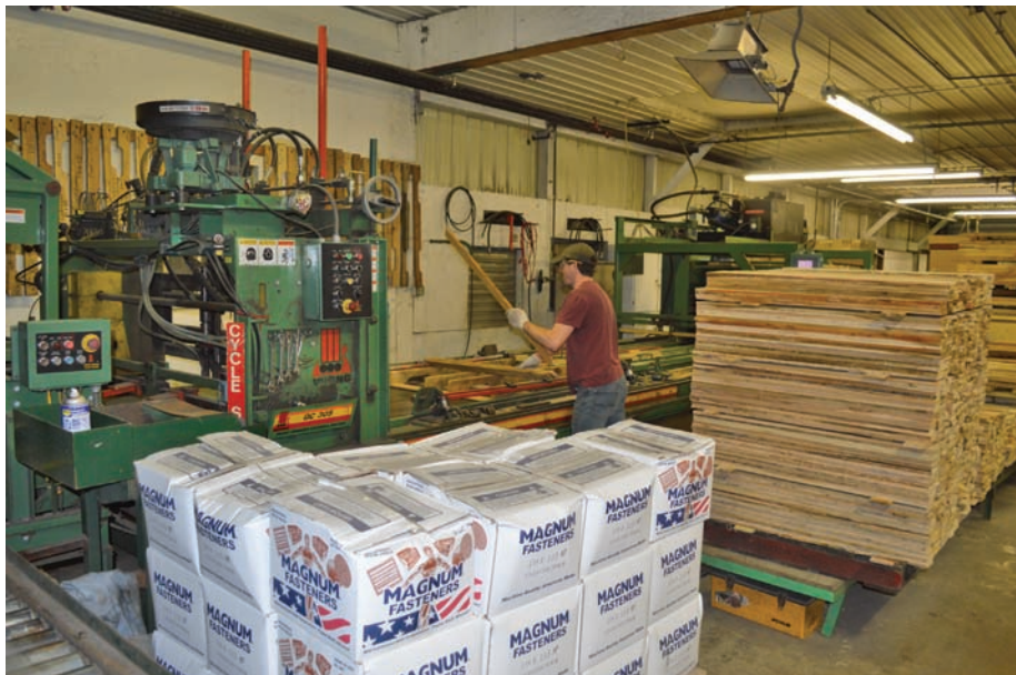
Mt. Eaton manufactures pallets on six Viking Champion nailing systems. They like them for the pallet quality that comes from hand placement and inspection of each board. They also provide the flexibility to build more pallet specifications in a single shift. Mt. Eaton uses Mid Continent bulk nails, as illustrated here.
