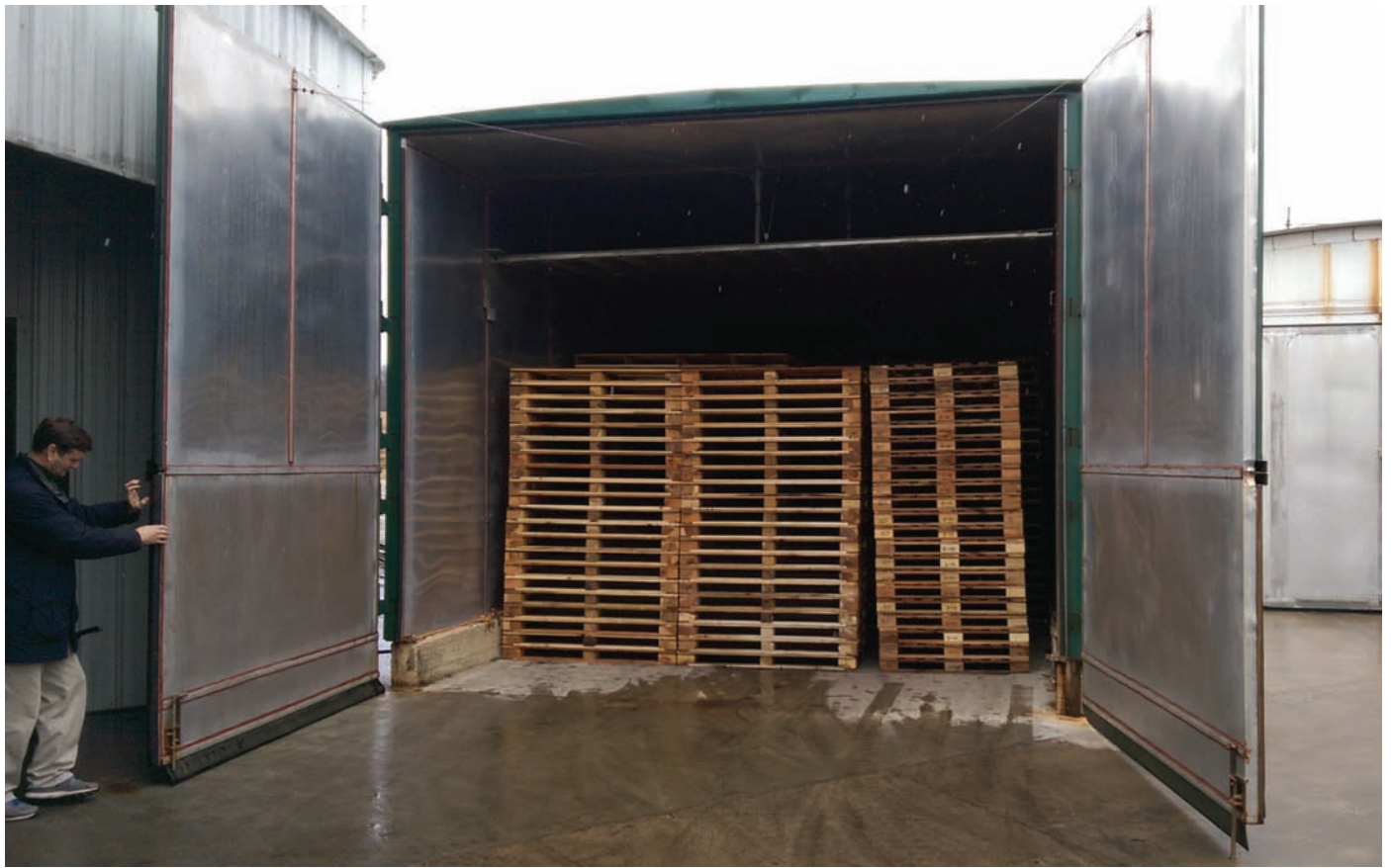
The new Kiln-Direct kiln features a greater fan capacity, hinged baffles for more efficient airflow, and a larger burner for more heat.
